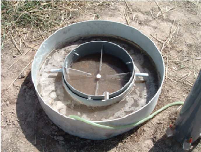
Figure 3. Photograph of field experiment setup, double-ring infiltrometer ( d_i = 40 cm, d_o = 70 cm).
